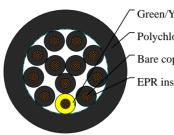
Green/Yellow wire Polychloroprene rubber outer jacket Bare copper conductor EPR insulation
